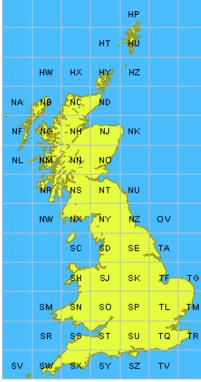
In each case the first half of the digits is for the first coordinate and the second half for the other. The most common form is the *six figure grid reference*, with three digits in each coordinate to determine a 100 m square. (Grid references are often be written with or without spaces, e.g. also **NZ631231**.)
